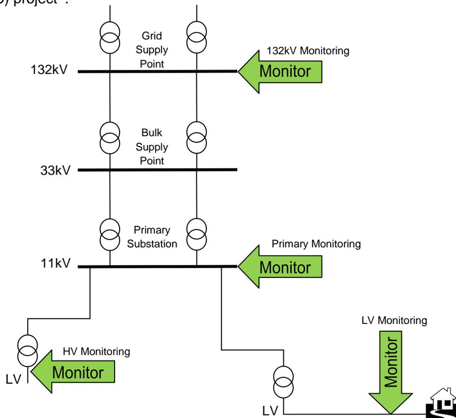
Figure 1: Illustration of CLASS monitoring requirements
