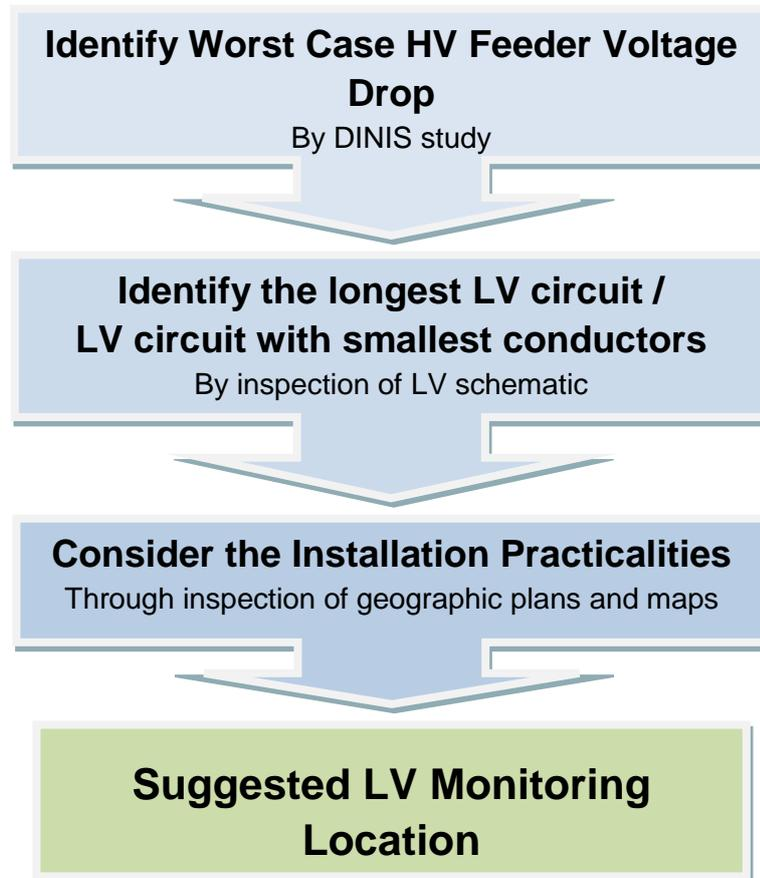
**Figure 2 :** LV Monitoring Location Selection Methodology
