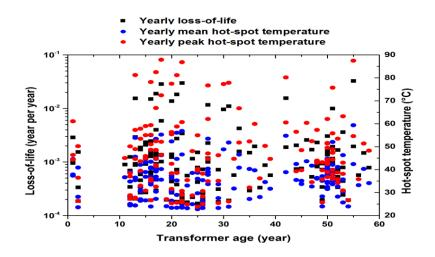
Figure 3.7: Yearly loss-of-life, mean and peak hot-spot temperatures under BAU scenario (No EVs penetration)
