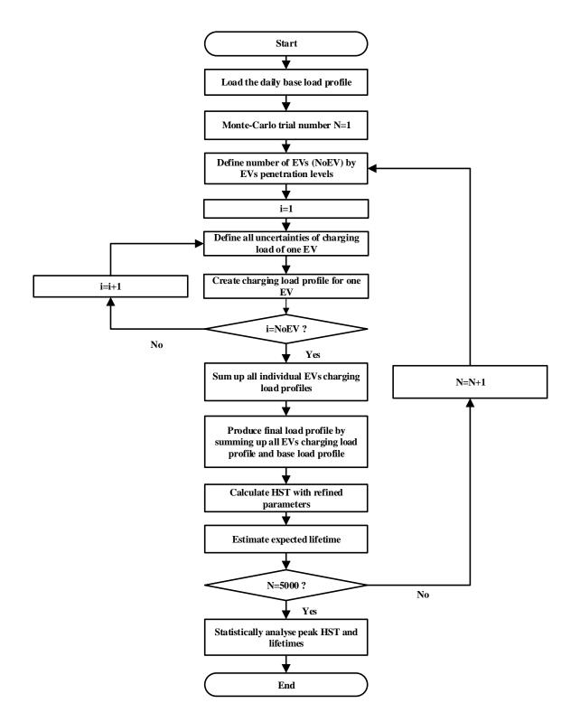
Figure 2.8: Flow chart of Monte-Carlo simulation to determine hot-spot temperature and lifetime of prototype distribution transformer under EV scenarios
