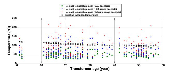
Figure 3.11: Peak hot-spot temperatures and bubbling inception temperatures under three EV scenarios
