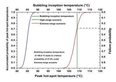
Figure 2.11: Example of determination of failure probability under EV scenarios
