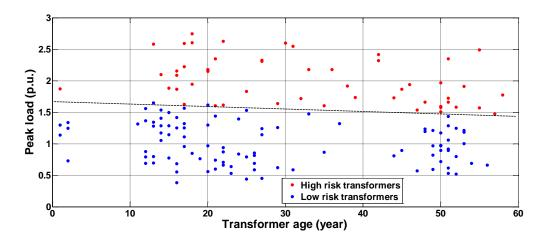
Figure 3.13: Comparison of peak loads between high risk transformers and low risk transformers under Extremerange scenario
