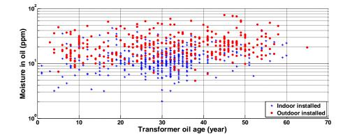
Figure 3.3: Corrected moisture data of indoor and outdoor installed distribution transformers
