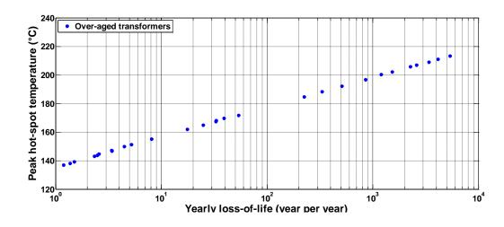
Figure 3.9: Peak hot-spot temperatures of over-aged distribution transformers
