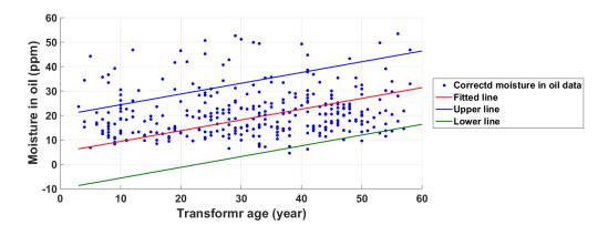
Figure 3.5: Fitting of moisture in oil data of outdoor distribution transformers
