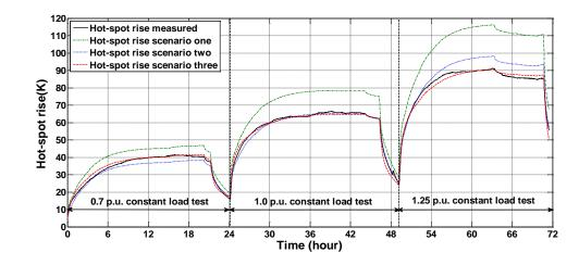
Figure 2.3: Calculated hot-spot temperatures with thermal parameters refined by two methods under heat run test loads
