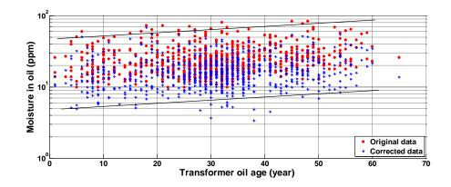
Figure 3.2: Originally measured moisture in oil data and corrected values of distribution transformer population
