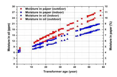
Figure 3.10: Moisture in oil and paper of selected transformers
