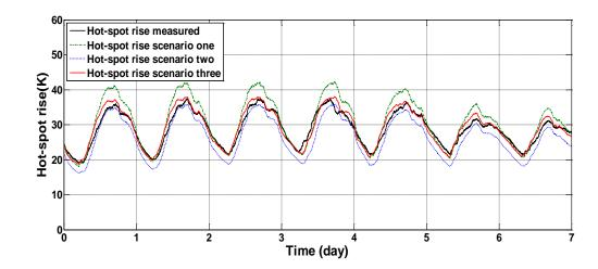
Figure 2.4: Calculated hot-spot temperatures with thermal parameters refined by two methods under cyclic loads
