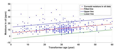
Figure 3.4: Fitting of moisture in oil data of indoor distribution transformers
