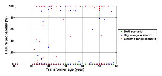
Figure 3.12: Failure probability under three EV scenarios
