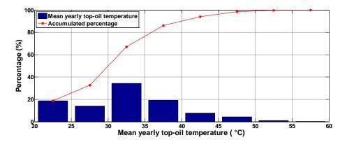
Figure 3.1: Mean yearly top-oil temperature of distribution transformer population calculated with Elexon profiles
