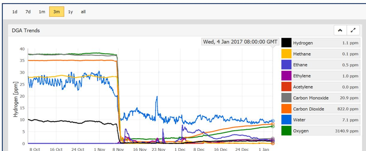
Continuing analysis of the transformer revealed that the DGA trends continued to remain at low levels validating that the oil regeneration process was successful.
