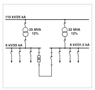
Figure 9:  $I_s$ -limiter in a bus section
