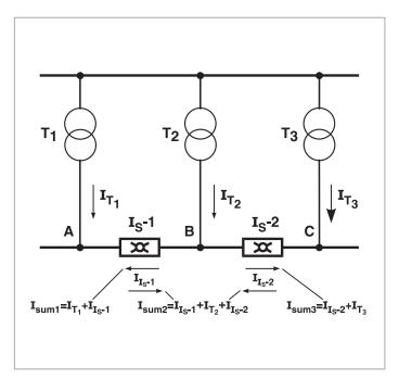
Figure 12: Schematic diagram-I<sub>s</sub>-limiter with summation of currents
