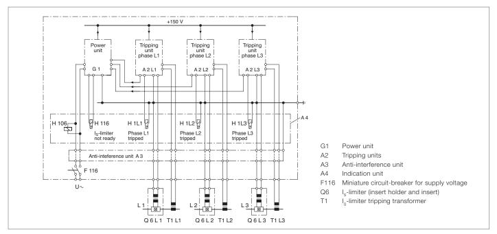
Figure 4: Schematic diagram of the Is-limiter equipment
