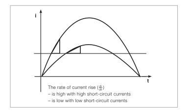
9. How does the I<sub>s</sub>-limiter distinguish between minor and serious short-circuits?
