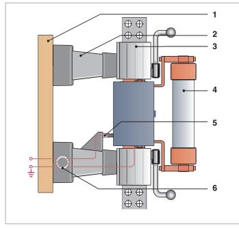
Figure 1: I<sub>s</sub>-limiter insert holder with insert for 12 kV, 2000 A
