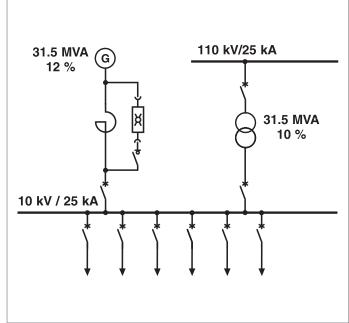
Figure 10: I<sub>s</sub>-limiter in connecting point with a public supply network
