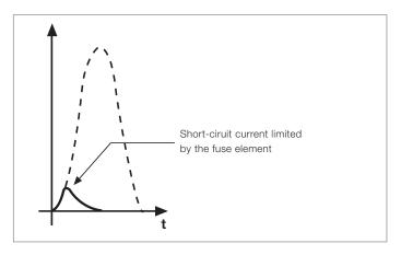
Does the I<sub>s</sub>-limiter trip on every short-circuit? No! The I<sub>s</sub>-limiter only trips when the system is at risk. Small short-circuit currents are interrupted by the circuit-breakers.
