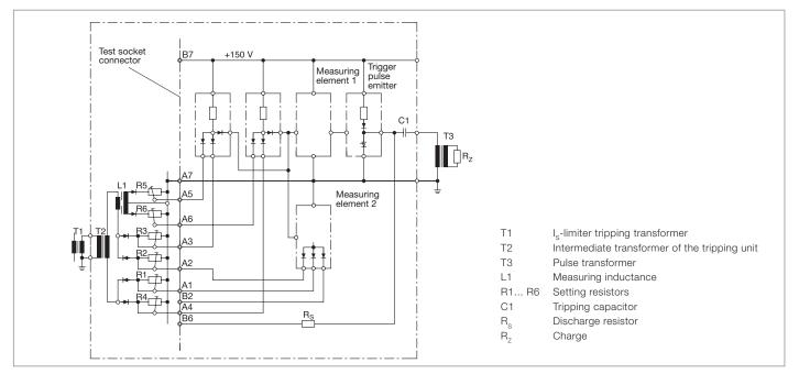
Figure 5: Schematic diagram of a measuring and tripping unit
