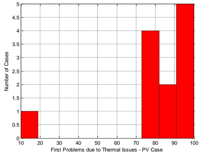
First Penetration Level with Technical Problems – PV Case
