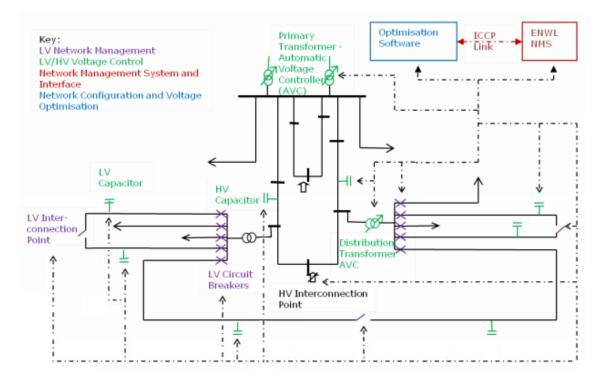
The LV network control will be established using new retrofit LV vacuum circuit breaker, WEEZAP and retrofit remote control link box switch, LYNX. Deploying the WEEZAP in conjunction with the LYNX will allow LV network interconnection and facilitate dynamic reconfiguration either locally or remotely from Electricity North West's Control Room. Where a link box does not exist at a proposed interconnection point then a new link box will be installed to allow the reconfiguration capability.
