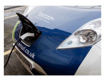
Research suggests that the charging behaviour of current EV users is to charge their EV for three hours every two days. Therefore most of the chargers we will install are slow (suitably designed and rated outdoor 13amp sockets) which will meet the charging needs of the majority of our colleagues.
